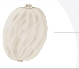
Economical grease pillows designed to fit into factory exhaust fan drip trays. Manufactured using recycled hydrophobic materials and bio-degradable grease neutralizers, so it only retains grease and lets water pass through. Retains up to 8x its weight in grease. An economical and effective solution where changing grease containment systems is not wanted.
