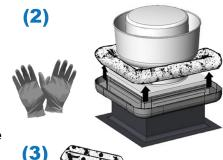
6) Reinstall the four Grease Gutter corners.
